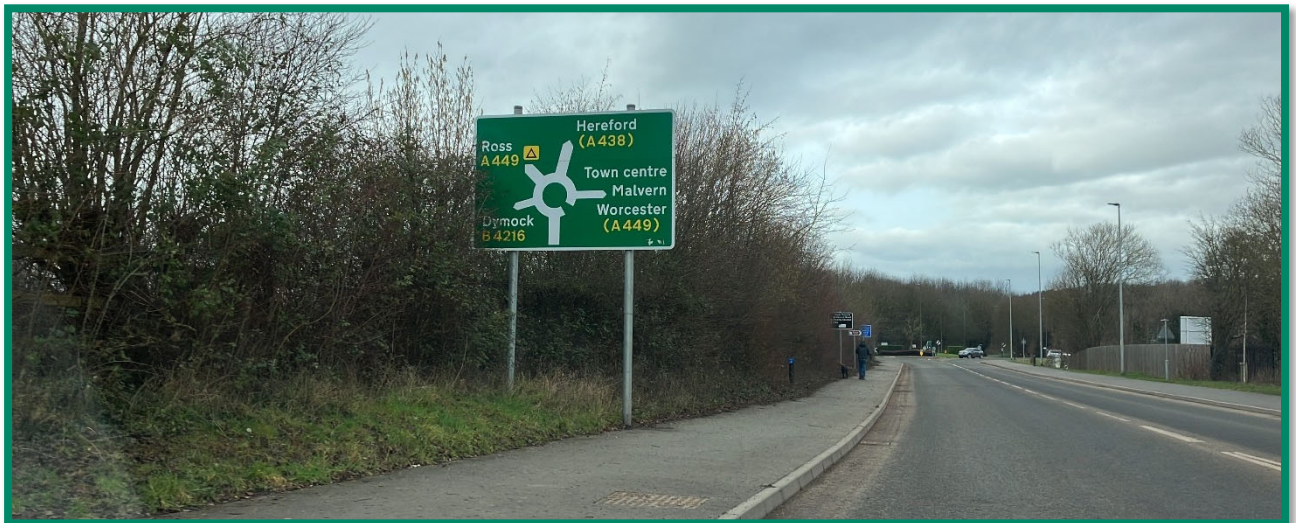
Figure 15 - Existing traffic sign located on the westbound approach to the A449 Leaddon Way/A449 Ross Road roundabout. The sign could be replaced if weight limit introduced on New Street, showing weight limit roundel associated with Town centre. Alternatively existing sign shown in Figure 18 is removed and replaced with a new map type sign showing the HGV routes to the industrial areas and weight limit on New Street.
