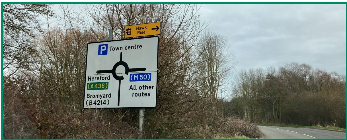
Figure 29 - Existing traffic sign located on Little Marcle Road approach to the Leadon Way/Lower Road roundabout. The sign could be replaced if weight limit introduced on Lower Road, showing weight limit roundel associated with Town centre.
