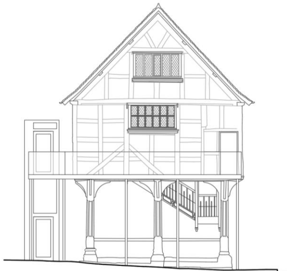
Fig F: North elevation with Stannah external platform lift
